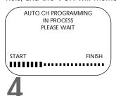
Wait for a few minutes while the VCR sets up the channels. When this is complete, CHANNELS ARE SET will appear on the screen. Then the programming of the lowest channel number placed in the VCR's memory will appear on the screen. Now when you press the CH(annel)  $\blacktriangle$ / $\checkmark$  buttons, you will scan only through channels you receive. You may still select non-memorized channels by pressing the Number buttons.
